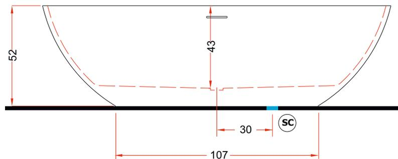
Scarico a terra consigliato Ø40mm. **SC** Recommended grounded drain Ø40mm.
